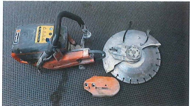
Cutting disc that came loose from the concrete saw
