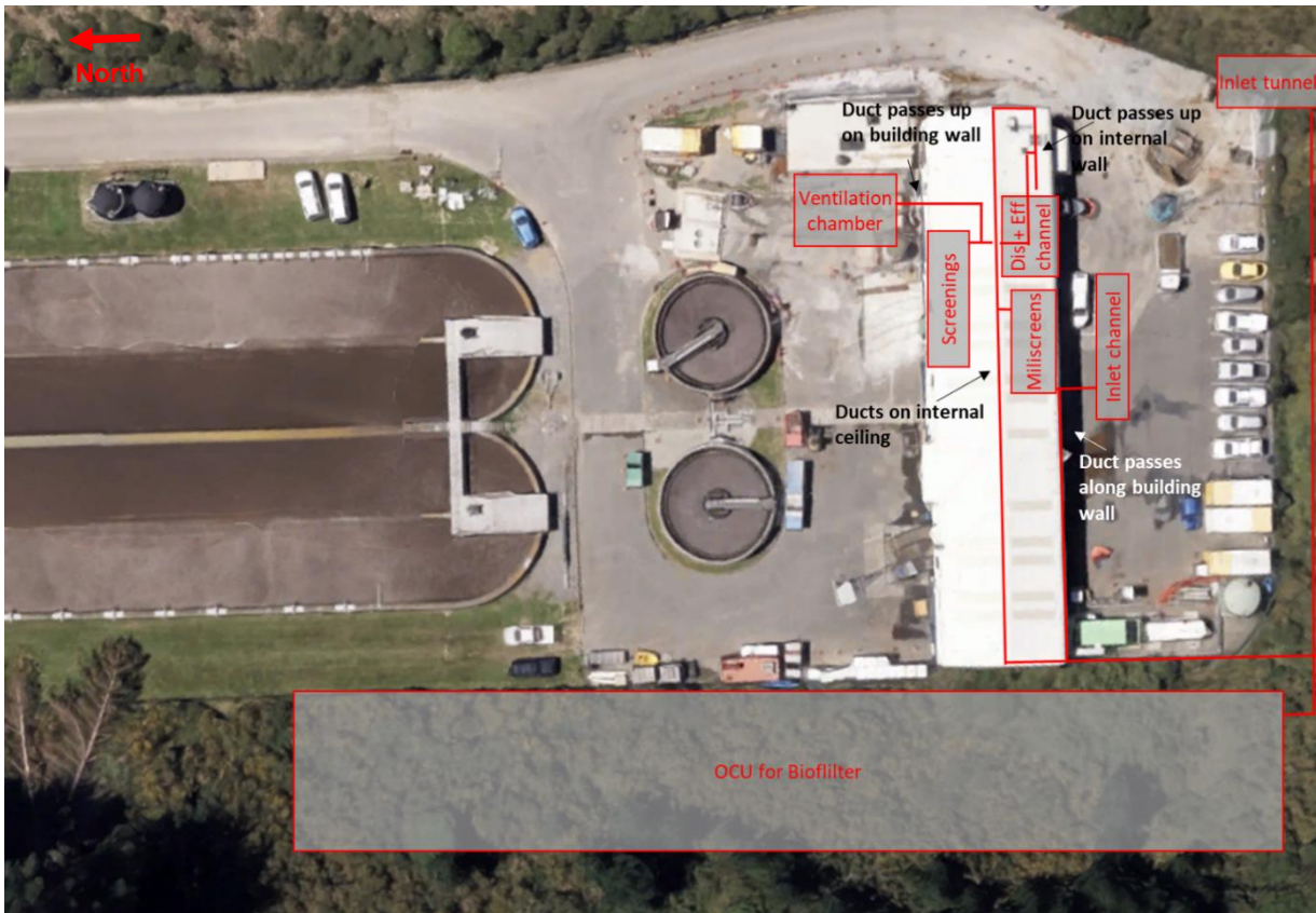
Figure 3-8: Ductwork arrangement for Biofilter OCU for Option 1
