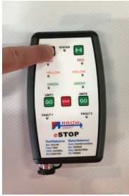
Switch on handset by holding the power button for 5 seconds
