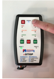
Switch to operation mode by holding the activation button for 5 seconds
