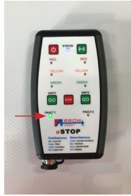
A green light will show once handset is connected to the lantern, this will happen automatically if it has been previously paired (see page 17)
