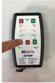
Press the go button to perform a lantern test. Each lantern will light for 0.5 seconds
