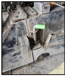
These spring-loaded pin locks should automatically drop when the hinge guard is placed in its operating position and require pulling up and releasing for the hinge guard to be lifted.
