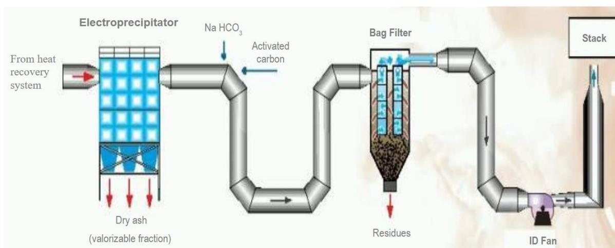
Figure 12: Typical Dry Treatment for Flue Gas
