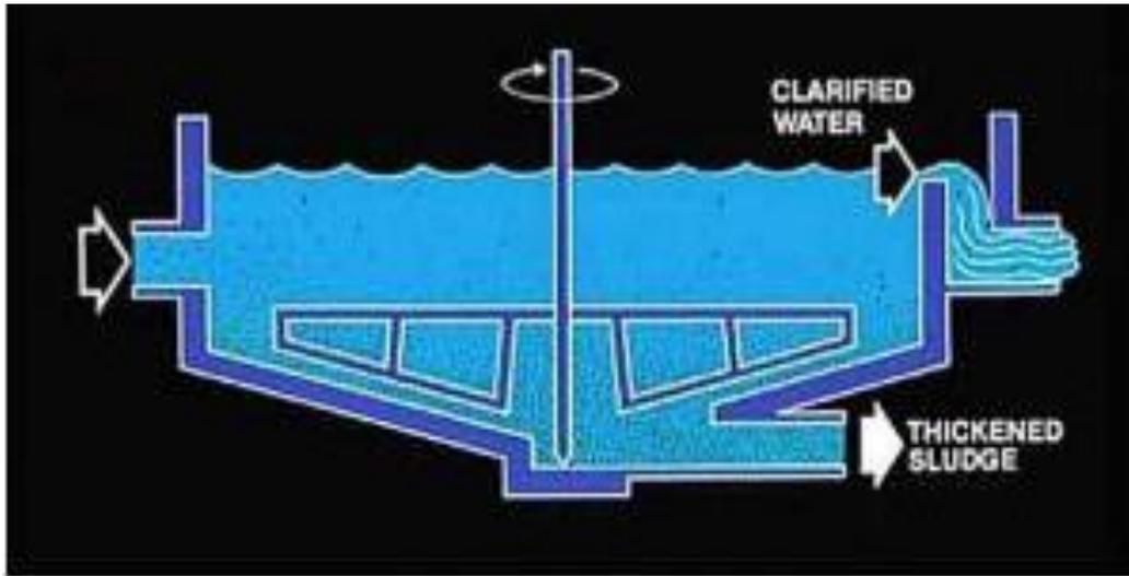
Figure 1: Schematic of a Static Gravity Thickener
