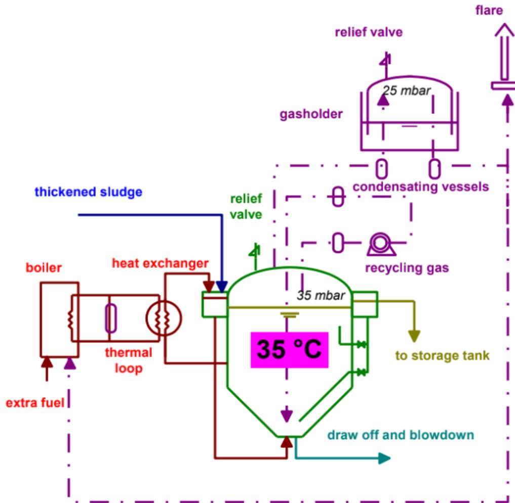
Figure 7: Schematic of a Mesophilic Anaerobic Digester
