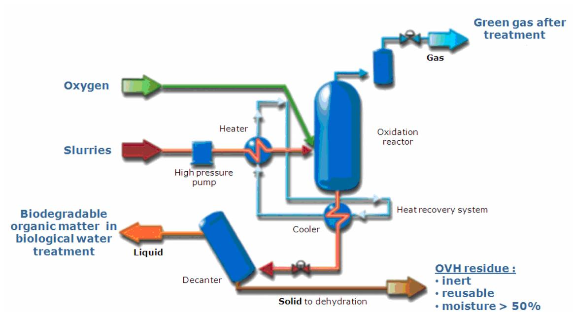
Figure 13: Schematic of the Wet Air Oxidation Process
