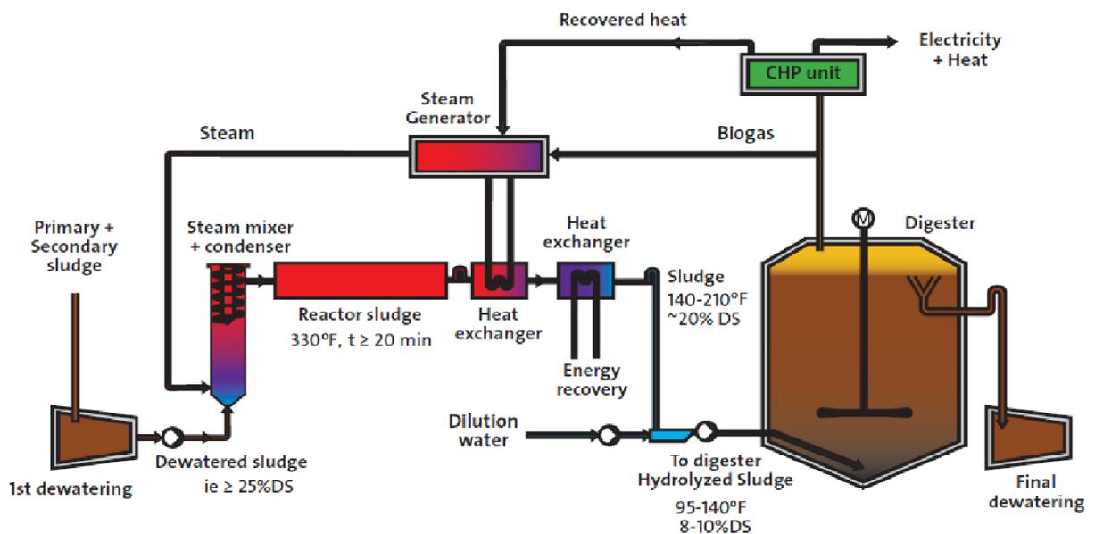
Figure 10: Schematic of a Continuous Thermal Hydrolysis Process
