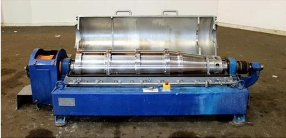
Figure 4: Example of Solid Bowl Centrifuge.
