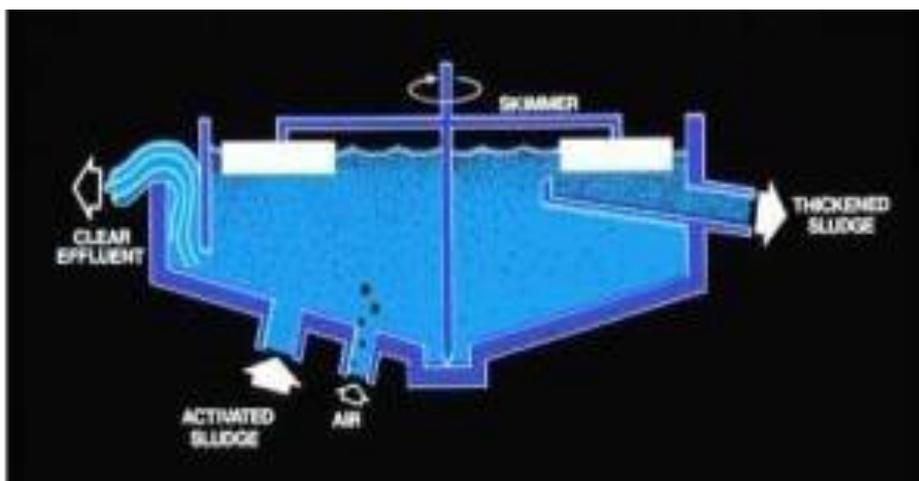
Figure 3: Schematic of a Dissolved Air Flotation Apparatus
