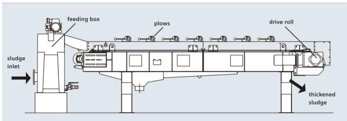
Figure 2 Schematic of a Gravity Belt Thickener
