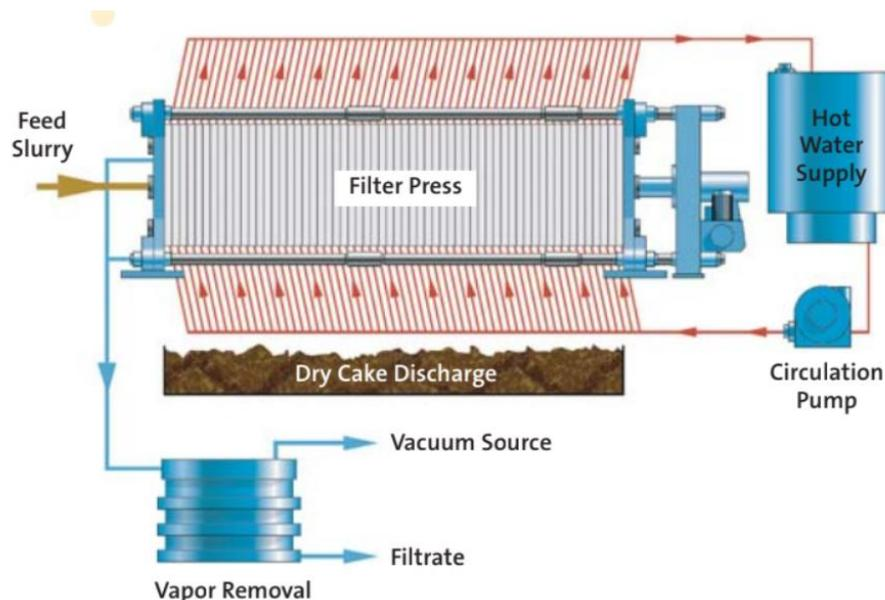
Figure 5: Schematic of a Heated Filter Press
