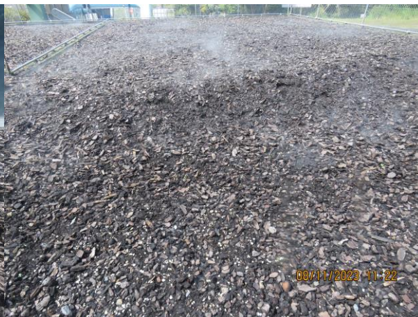
Figure 2: Cell 1 Smoke Test, 8 November 2023 Short Circuiting, 8 November 2023
