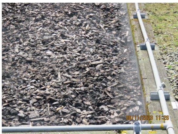
Figure 4: Cell 2 Smoke Test Short Circuiting, 8 November 2023
