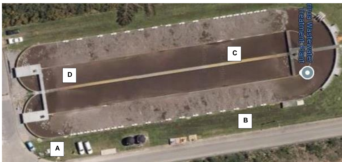
Figure 3 – Porirua WWTP Oxidation Ditch with Indicative Probes Locations
