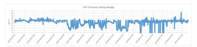
It has been observed that the UVT readings are not reliable and have fluctuated significantly since the 19th of September. The instrument supplier was on-site investigating, and they have recommended improvements such as installing the instrument in a horizontal position which might provide a more representative reading. Cleaning method based on air scouring was suggested as well. Adjustments as per recommendations are ongoing at the time of preparing this report.
