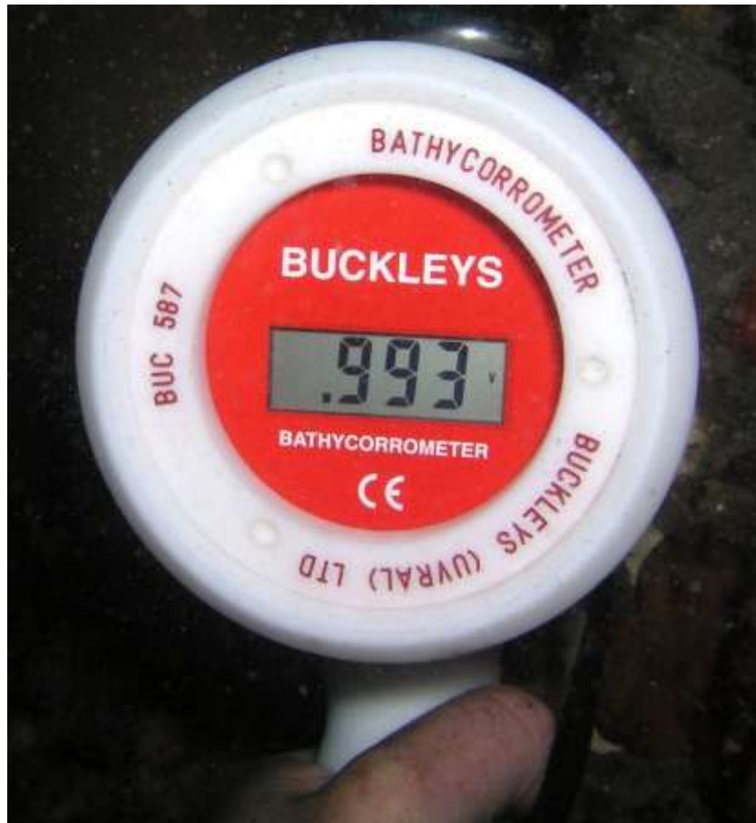
Figure 20: BCM (Cathodic Potential Meter) in operation
