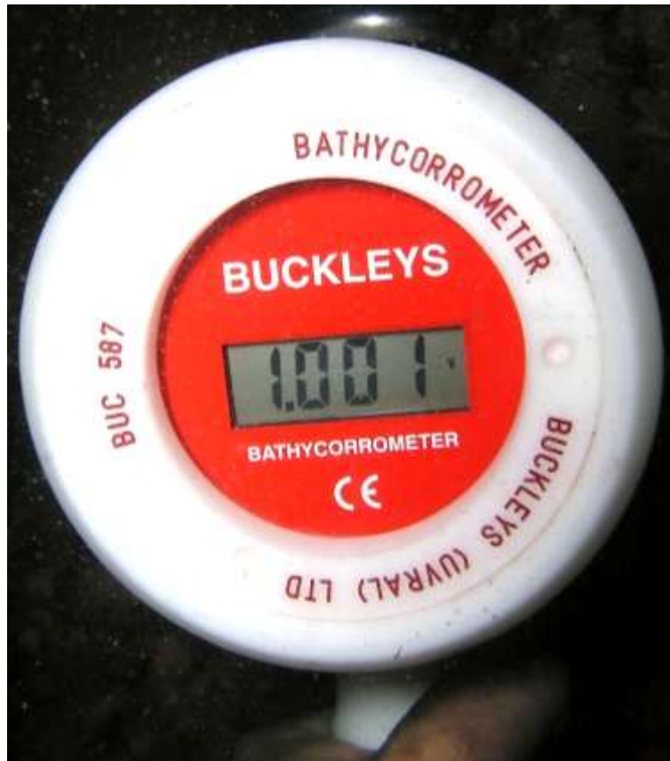
Figure 23: Cathodic Potential reading taken at Diffuser # 3
