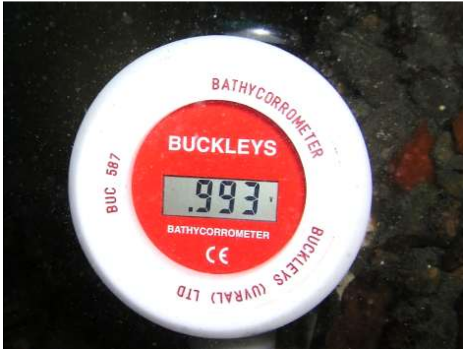
Figure 25: Cathodic Potential reading taken at Diffuser # 11
