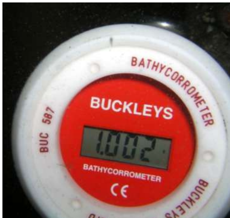
Figure 24: Cathodic Potential reading taken at Diffuser # 7
