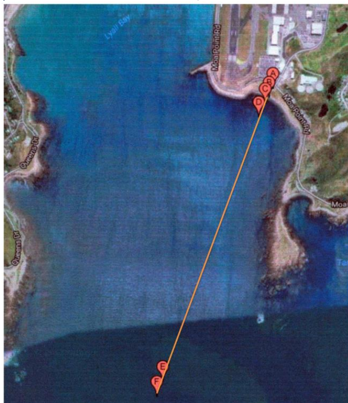
Figure 1, Pipeline route and key reference positions
