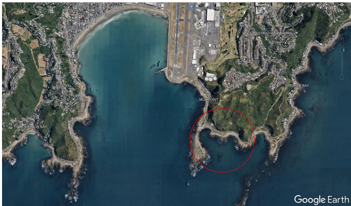
Figure 4-1: Location of the short outfall shown at centre of a 400m radius mixing zone (red circle)
