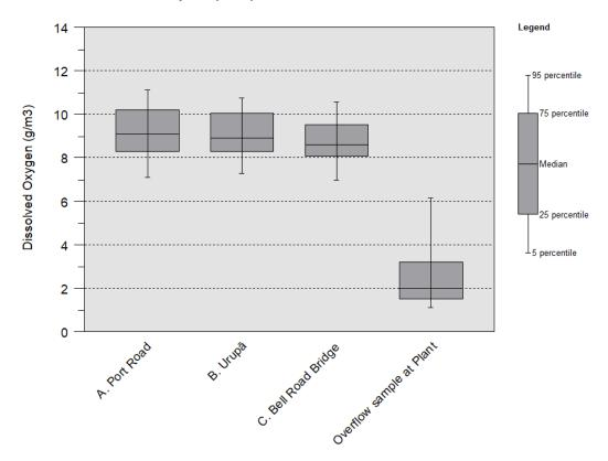
Figure 3-5 Box plot summary of dissolved oxygen<sup>6</sup> at Waiwhetu Stream site A, B and C and overflow sample at the wastewater treatment plant (N=41).
