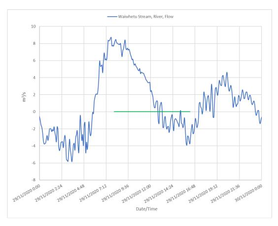
Figure 0-9: Flow at lower Waiwhetu Stream near the Seaview outfall during 29 November 2020 overflow event
