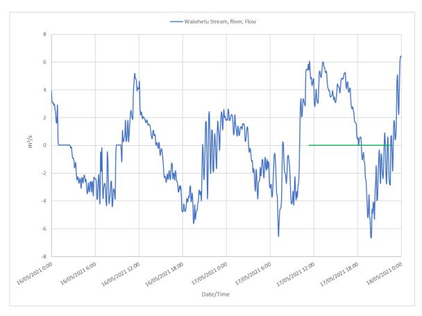
Figure 0-13: Flow at lower Waiwhetu Stream near the Seaview outfall during 17 May 2021 overflow event
