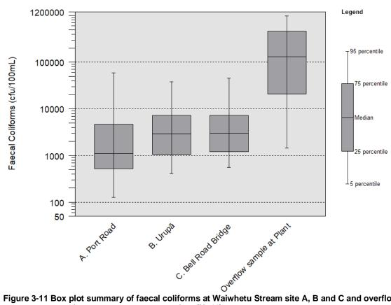
Figure 3-11 Box plot summary of faecal coliforms at Waiwhetu Stream site A, B and C and overflow sample at the wastewater treatment plant (N=41).
