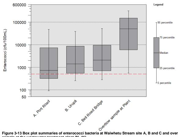
Figure 3-13 Box plot summaries of enterococci bacteria at Waiwhetu Stream site A, B and C and overflow sample at the wastewater treatment plant (N=41).
