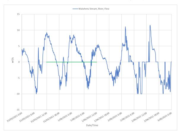
Figure 0-14: Flow at lower Waiwhetu Stream near the Seaview outfall during 31 May 2021 overflow event
