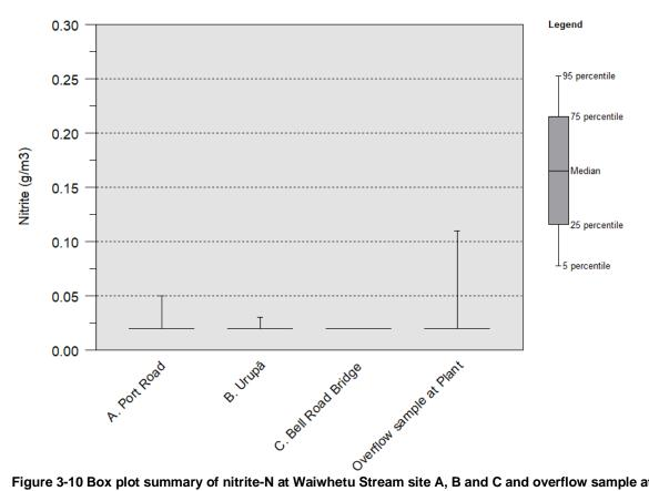
Figure 3-10 Box plot summary of nitrite-N at Waiwhetu Stream site A, B and C and overflow sample at the wastewater treatment plant (N=41).
