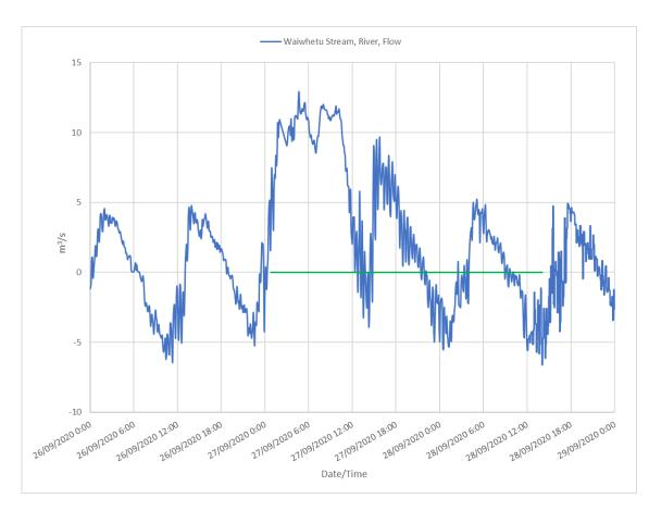
Figure 0-5: Flow at lower Waiwhetu Stream near the Seaview outfall during 27 September 2020 overflow event
