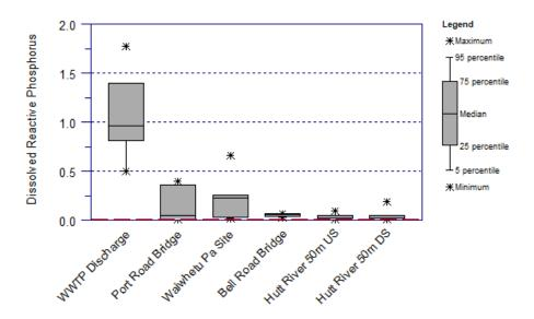
Figure 3-10: Box plot summary for dissolved reactive phosphorus (mg/L). ANZG DGV is shown as red line
