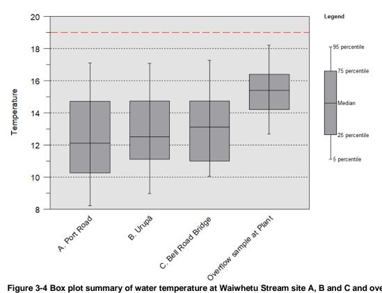
Figure 3-4 Box plot summary of water temperature at Waiwhetu Stream site A, B and C and overflow sample at the wastewater treatment plant (N=41).
