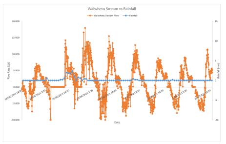
Figure 3-2: Waiwhetu Stream flow (L/s) in the tidal reach near the Seaview WWTP outfall
