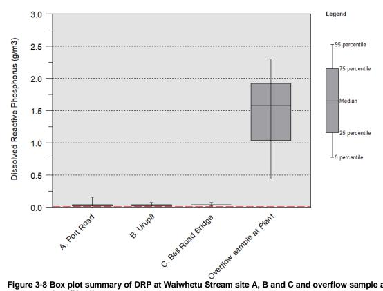
Figure 3-8 Box plot summary of DRP at Waiwhetu Stream site A, B and C and overflow sample at the wastewater treatment plant (N=41).
