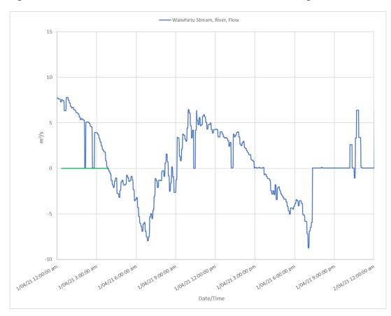
Figure 0-12: Flow at lower Waiwhetu Stream near the Seaview outfall during 1 April 2021 overflow event
