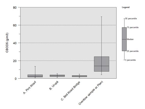
Figure 3-6 Box plot summary of CBOD<sub>5</sub> at Waiwhetu Stream site A, B and C and overflow sample at the wastewater treatment plant (N=41).
