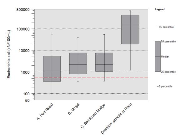
Figure 3-12 Box plot summaries of E.coli at Waiwhetu Stream site A, B and C and overflow sample at the wastewater treatment plant (N=41).
