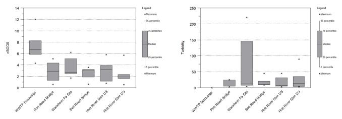
Figure 3-6: Box plot summaries of carbonaceous cBOD<sub>5</sub> (mg/L) and turbidity (NTU) results
