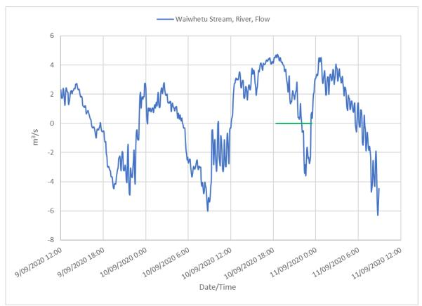
Figure 0-2: Flow at lower Waiwhetu Stream near the Seaview outfall during 10 September 2020 overflow event
