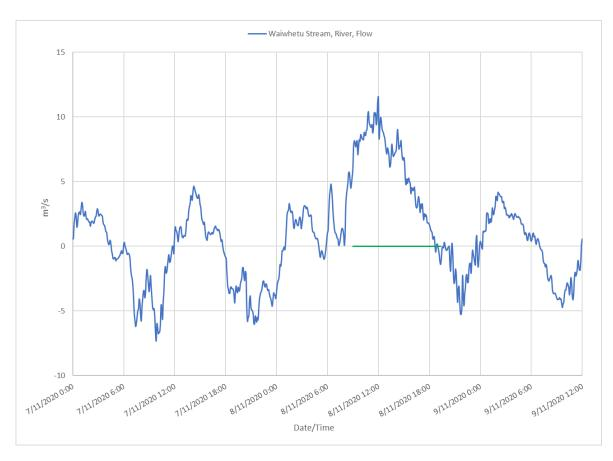
Figure 0-7: Flow at lower Waiwhetu Stream near the Seaview outfall during 8 November 2020 overflow event
