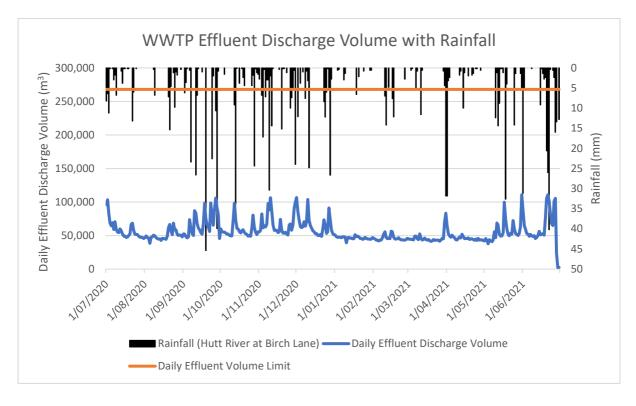
Figure 1: WWTP Effluent Flow Summary
