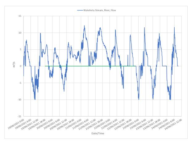
Figure 0-15: Flow at lower Waiwhetu Stream near the Seaview outfall during 19 June 2021 overflow event
