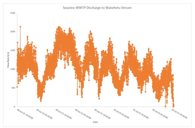
Figure 3-3: Seaview WWTP discharge to Waiwhetu Stream (L/s)
