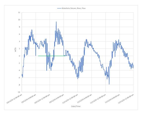
Figure 0-11: Flow at lower Waiwhetu Stream near the Seaview outfall during 10 December 2020 overflow event
