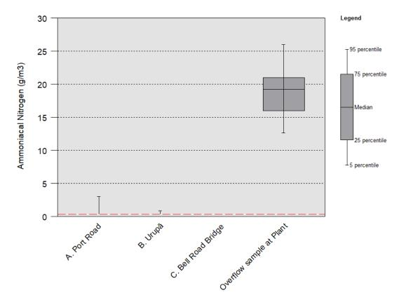
Figure 3-7 Box plot summary of ammoniacal-N at Waiwhetu Stream site A, B and C and overflow sample at the wastewater treatment plant (N=41).
