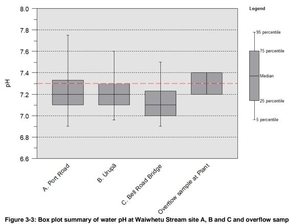
Figure 3-3: Box plot summary of water pH at Waiwhetu Stream site A, B and C and overflow sample at the wastewater treatment plant (N=41).
