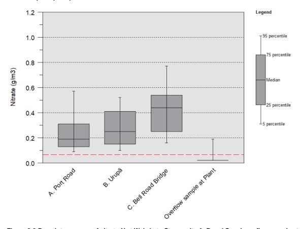
Figure 3-9 Box plot summary of nitrate-N at Waiwhetu Stream site A, B and C and overflow sample at the wastewater treatment plant (N=41).
