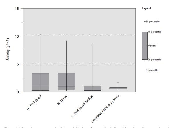
Figure 3-2 Box plot summary of salinity at Waiwhetu Stream site A, B and C and overflow sample at the wastewater treatment plant (N=41).
