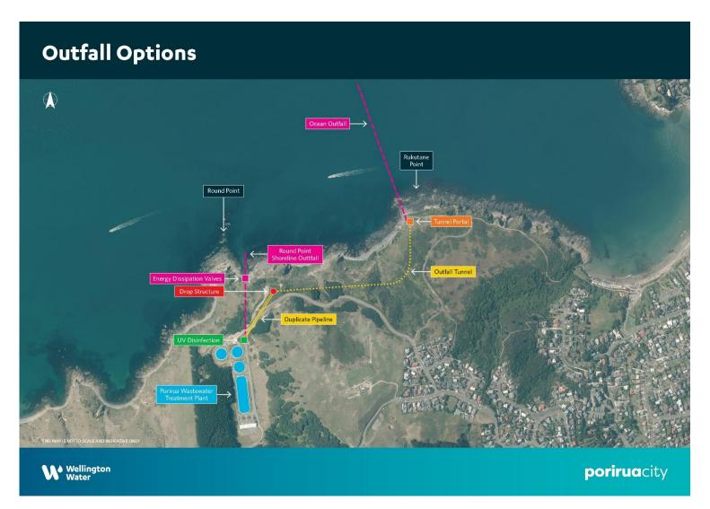
Figure 1., continued. Location of the alternative outfall options at Round Point (option 3) and offshore from the existing outfall (option 5b).
