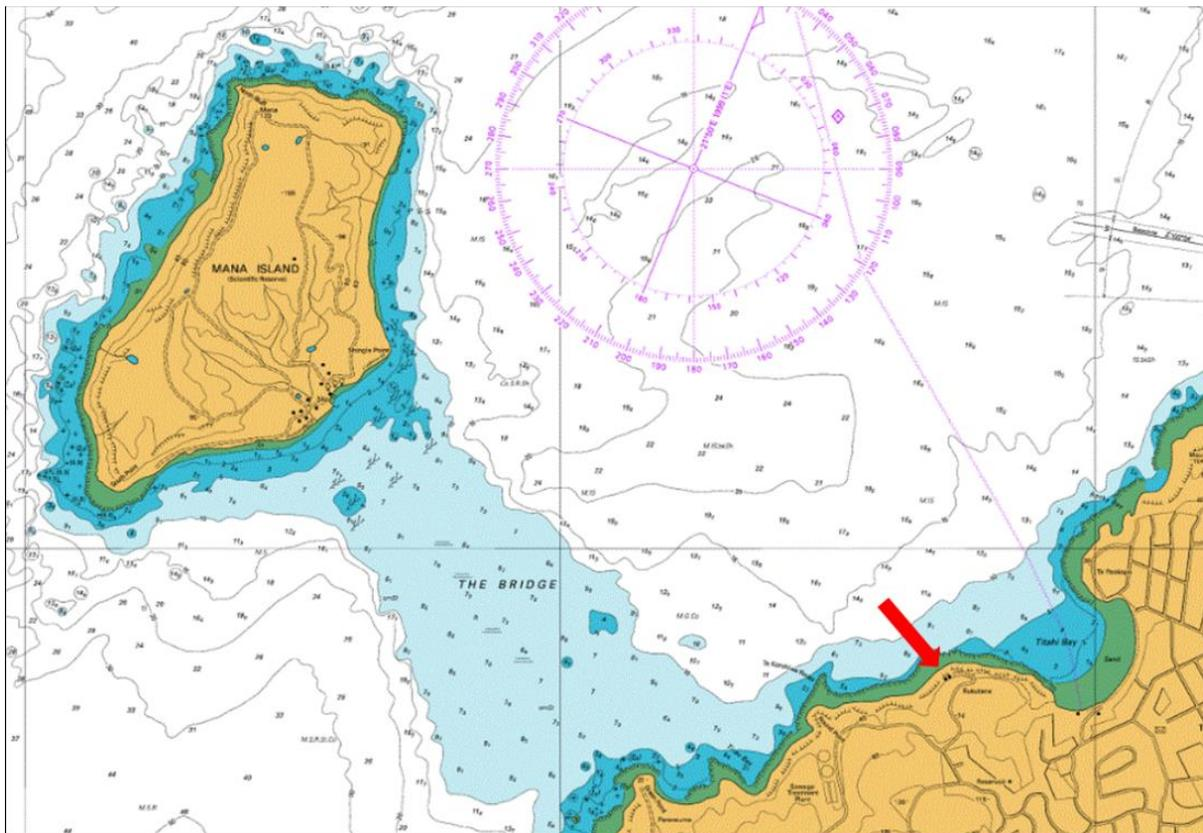
Figure 3. Detail from navigational chart NZ4632 showing the existing outfall of the Porirua WWTP (red arrow) and *The Bridge* between the mainland and Mana Island. Source: Land Information New Zealand (LINZ) and licenced by LINZ for re-use under the Creative Commons Attribution 4.0 International licence.
