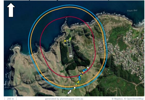
Figure 7: Odour intensity buffers showing the extent of odours from the plant
