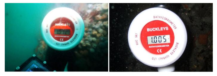
Figure 27: Diffuser # 10 port nozzle – 1.012mV Figure 28: Diffuser #
