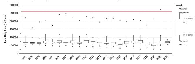
Figure 3-1: Total daily effluent flow rate from Moa Point WWTP (maximum permitted flow indicated by red line)
