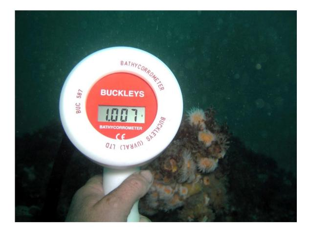
To protect a steel structure or installation in seawater, a more active metal than the steel is selected from the galvanic series and placed in contact with the steel below water level.
