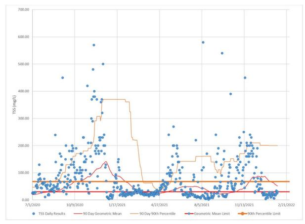
Figure 3-5: Daily treated wastewater TSS (mg/L), 90-day geometric mean and 90-day 90th percentile
