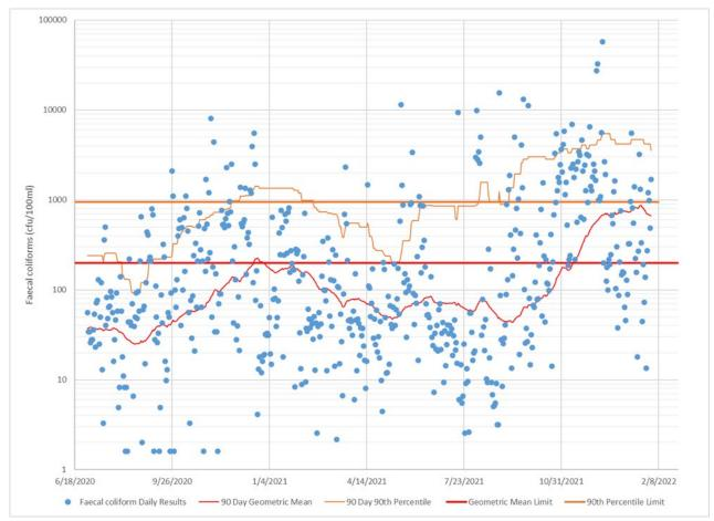
Figure 3-7: Summary of daily treated wastewater faecal coliform results (cfu/100ml) on a log scale
