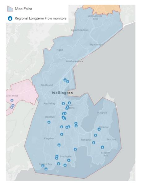
Figure 2 - Map of Active Wastewater Flow and Overflow Monitoring Sites within Moa Pt WWTP Catchment
