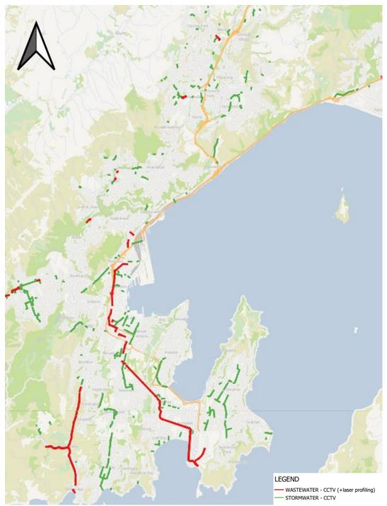
Figure 3 - Very High Critical Assets (VHCA) CCTV and laser profiling inspections completed as of June 2022.
