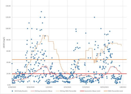
Figure 3-3: Daily treated wastewater cBOD5 (mg/L), 90-day geometric means and 90-day 90th percentiles
