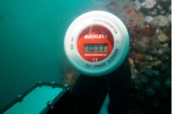
Figure 25: Diffuser # 1 test point – 1.024mV
