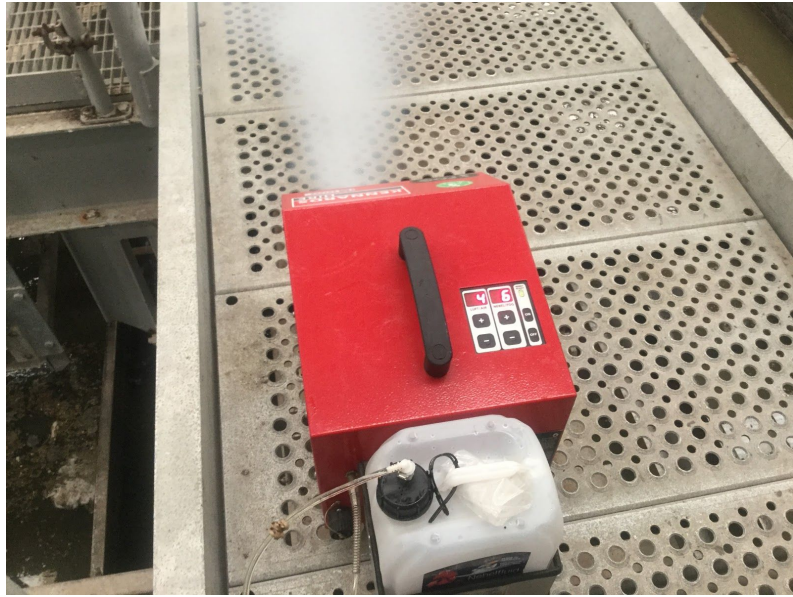
Smoke machine starting to saturate the Primary Tank area
