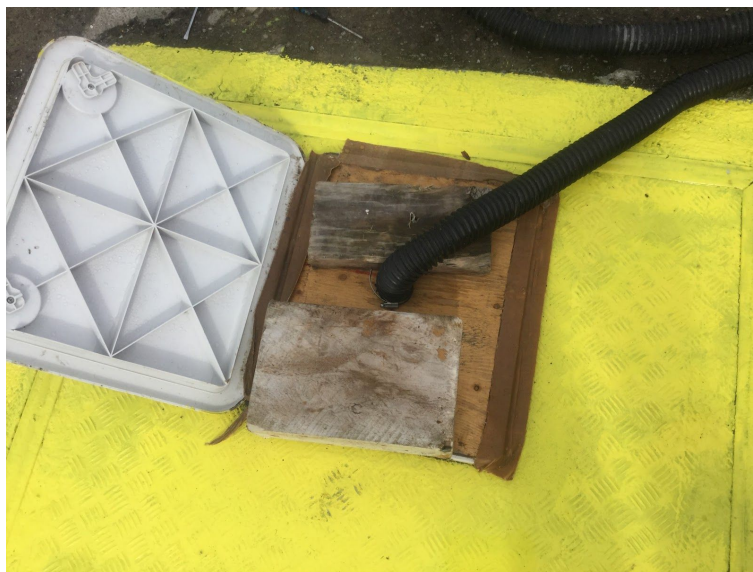
Smoke generator discharging into the inlet sampling chamber
