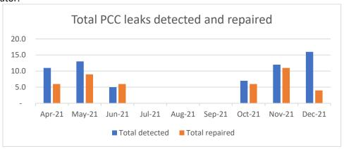
**Drinking Water Leakage Detection and Repair Process:** Using information from (existing) District Area Meters and (new) Small Area Monitors to automate Minimum Night Flows trends in various DMAs, and to establish, develop and document our end-to-end leak detection and repair process in Upper Hutt (as a Pilot), in order to identify areas for future improvements.
