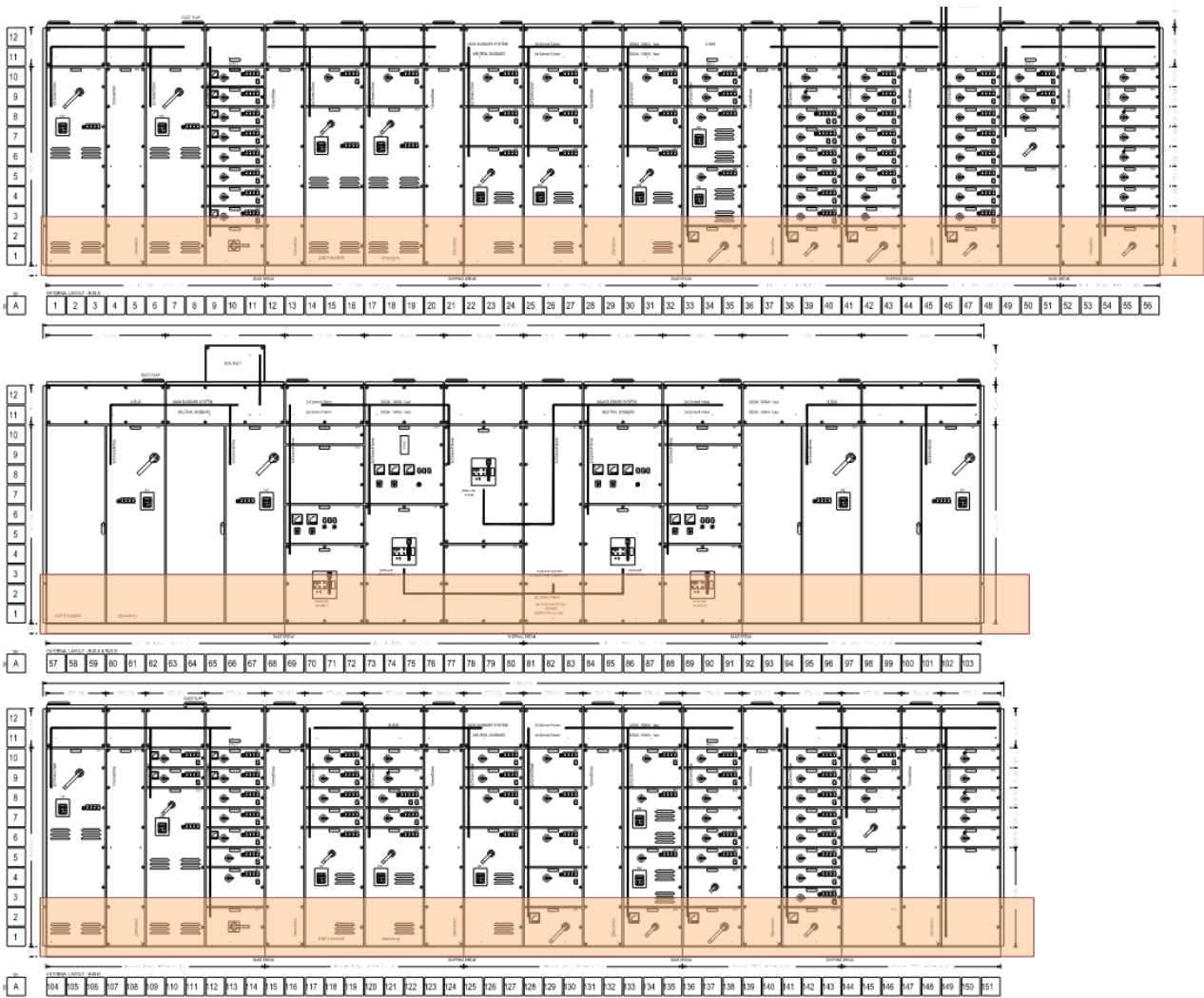
Figure 70: Indication of the approximate level to which MCCs were submerged
