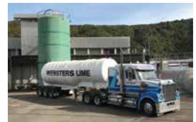
Our suppliers continued to provide the critical chemicals needed for water treatment and other services. Lime is used to adjust the pH, or acidity, of treated drinking water.
