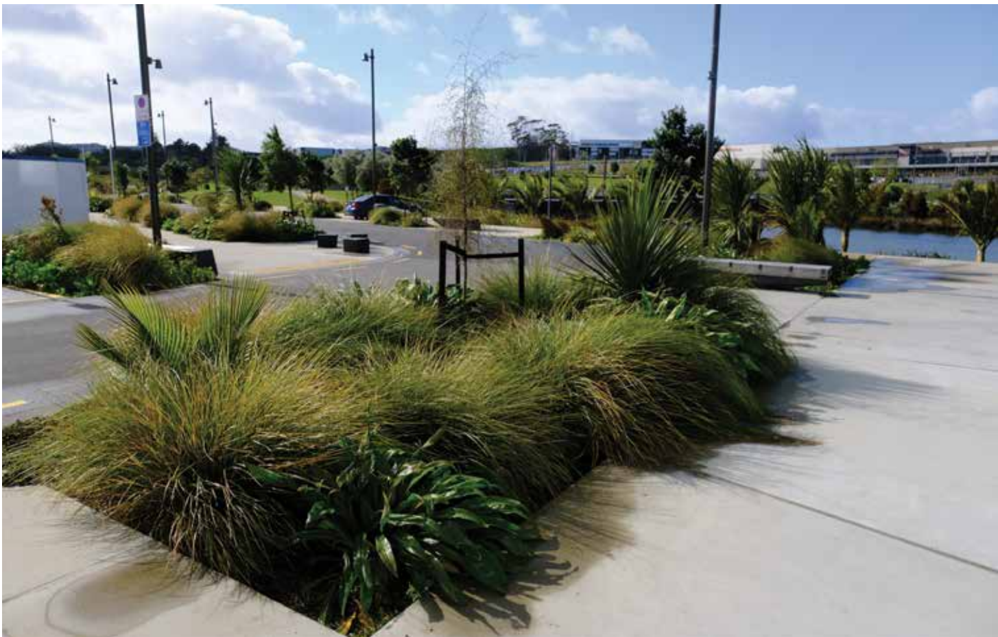
Green infrastructure harvests, cleans and recycle water, increases biodiversity, supports carbon sequestration and reduces urban heat island effects.
