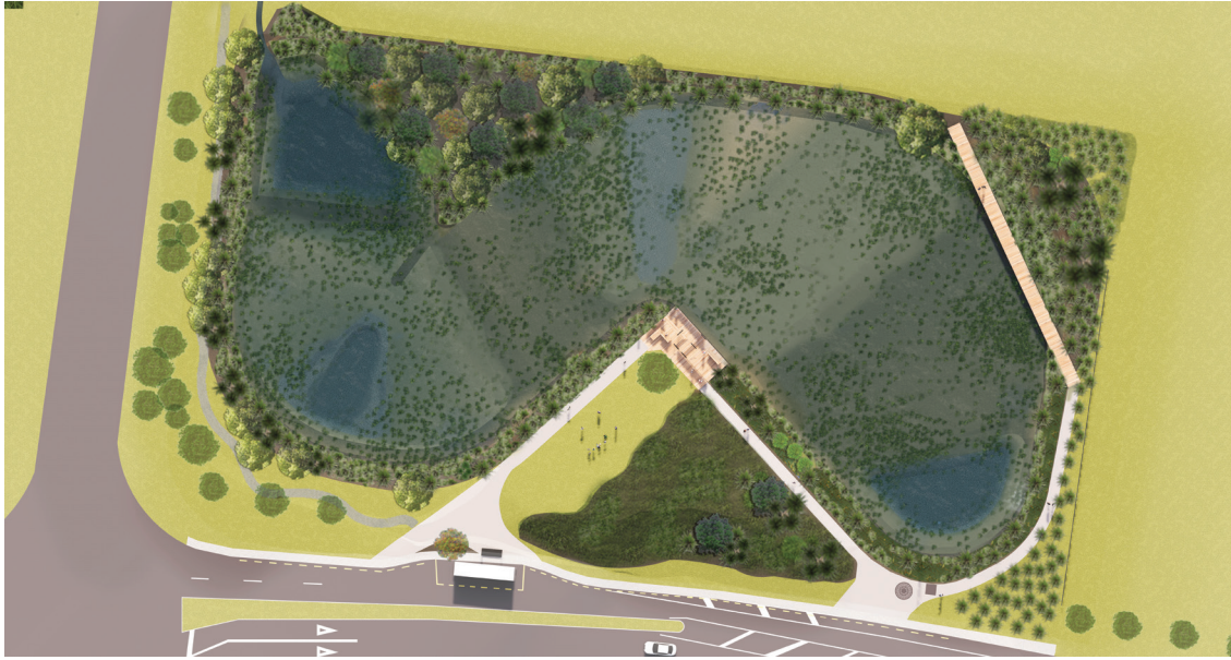
An overview of the Awarua wetland being constructed in Elsdon Park, Porirua. It will combine water sensitive urban design with large scale traditional infrastructure to greatly improve stormwater management.
