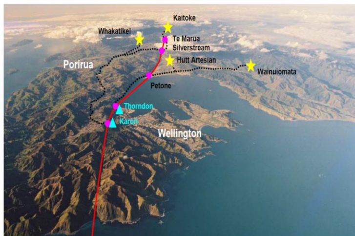
Bulk water network – several crossings over the fault
