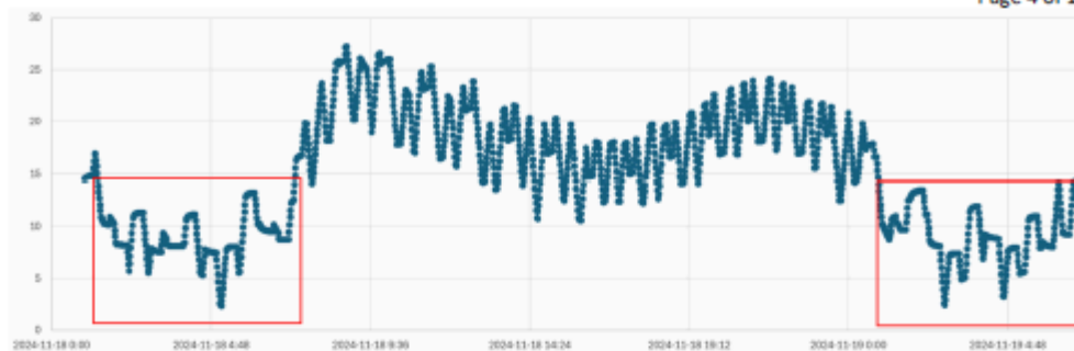
Figure 3 Diurnal flow profile from Rukutane Pump Station in L/s (shutdown hours indicated)
