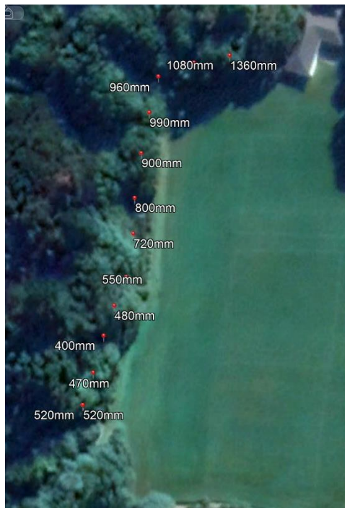
Figure 4 – Measurements from stream bed to crest of bund (stream flows from bottom (south) to top (north)) as at 30 July 2020.
