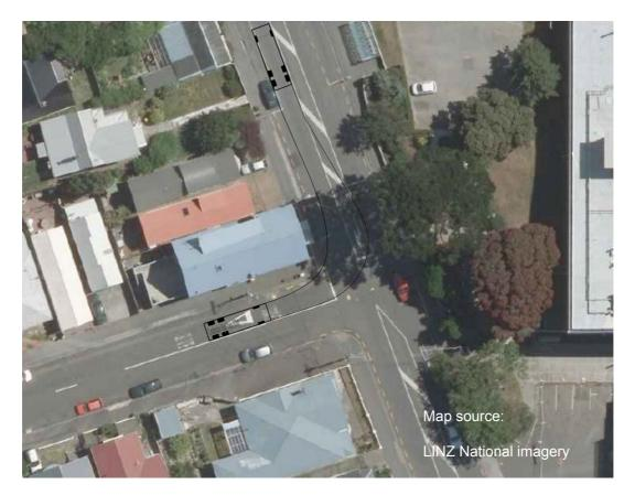
Figure 4-2: Rigid construction vehicle tracking curve. Left turn out of Rolleston Street
