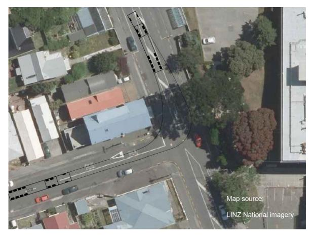
Figure 4-4: Articulated vehicle tracking curve. Left turn out of Rolleston Street
