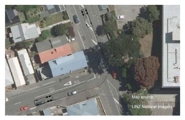
Figure 4-1: Rigid construction vehicle tracking curve. Right turn into Rolleston Street
