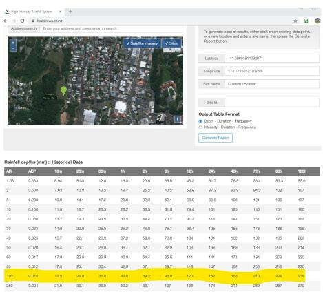
The 100yr ARI (AEP 0.01) for 10mins is 18.5mm. 3000m<sup>2</sup> x 0.018m = 54m<sup>3</sup>
