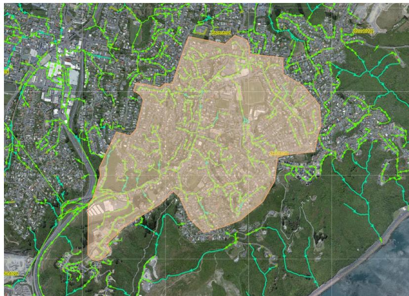
In addition to the private inspections, we will be doing a CCTV inspection of the public wastewater network. The inspection will be staged over the next two financial years. The pipes to be inspected are highlighted below.
