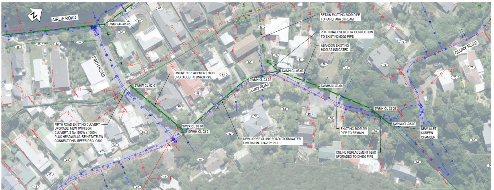
UPPER CLUNY ROAD STORMWATER DIVERSION PIPELINE PLAN
