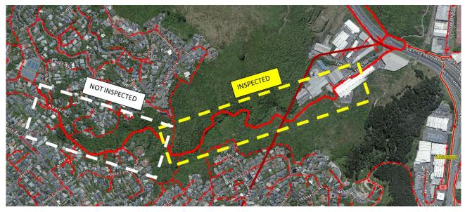
Prior to the site inspection walkover dye was introduced into the wastewater network using standard drainage dye, the purpose of this is that any leak in the wastewater pipe in close proximity to the stream would leak dye and would be identified through colouration of the stream. No dye was identified in the stream or leaking from wastewater pipe during the inspection. A map of where dye was introduced prior to the inspection is shown below.
