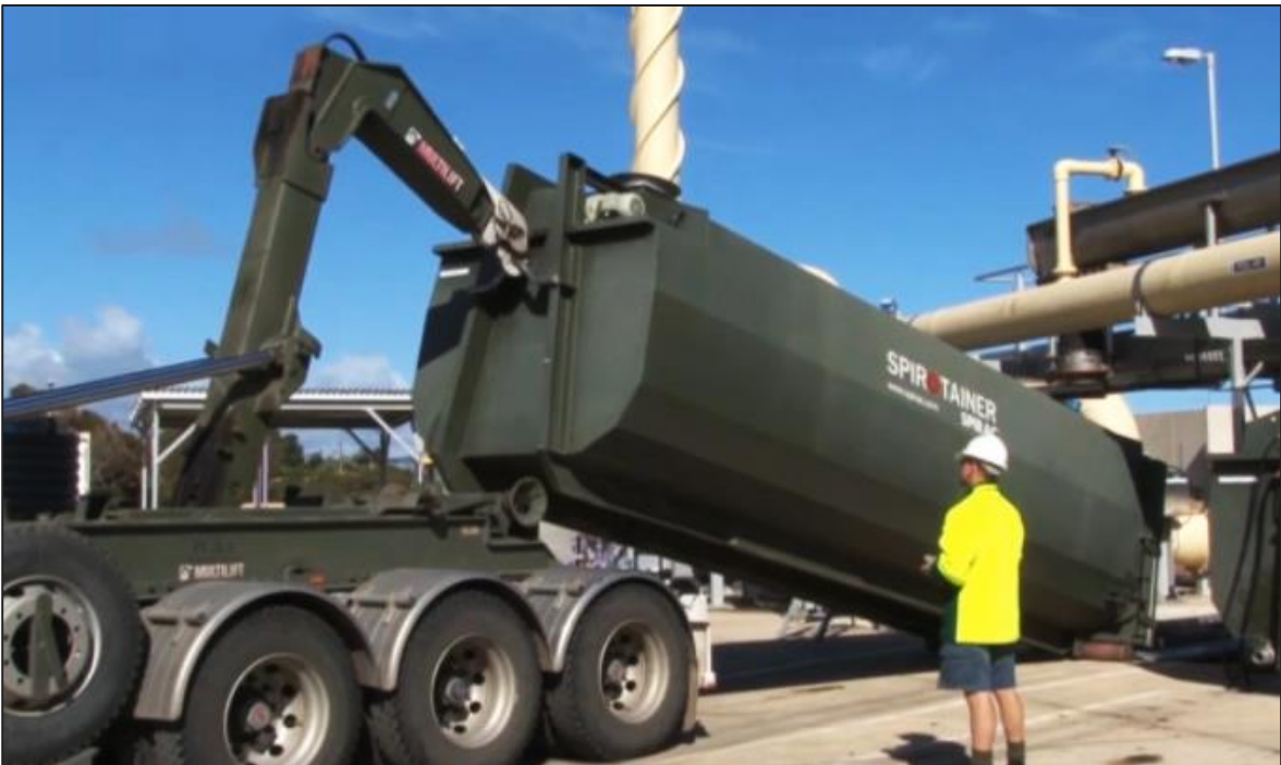
Figure 14 Self Levelling Bin Loading onto Hooklift Truck (Spirac Spirotainers®)
