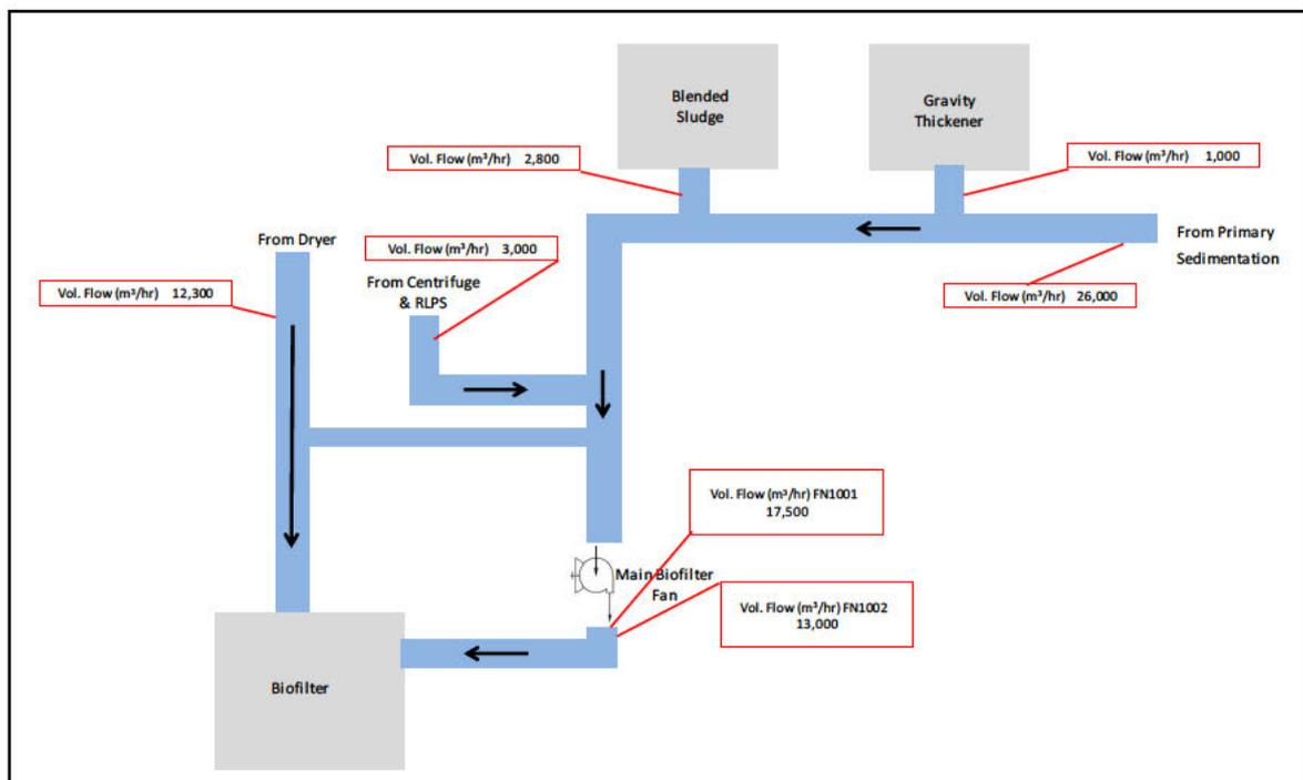
■ **Figure 11: Biofilter Total Extraction Rate Schematic, 24 February 2023**
