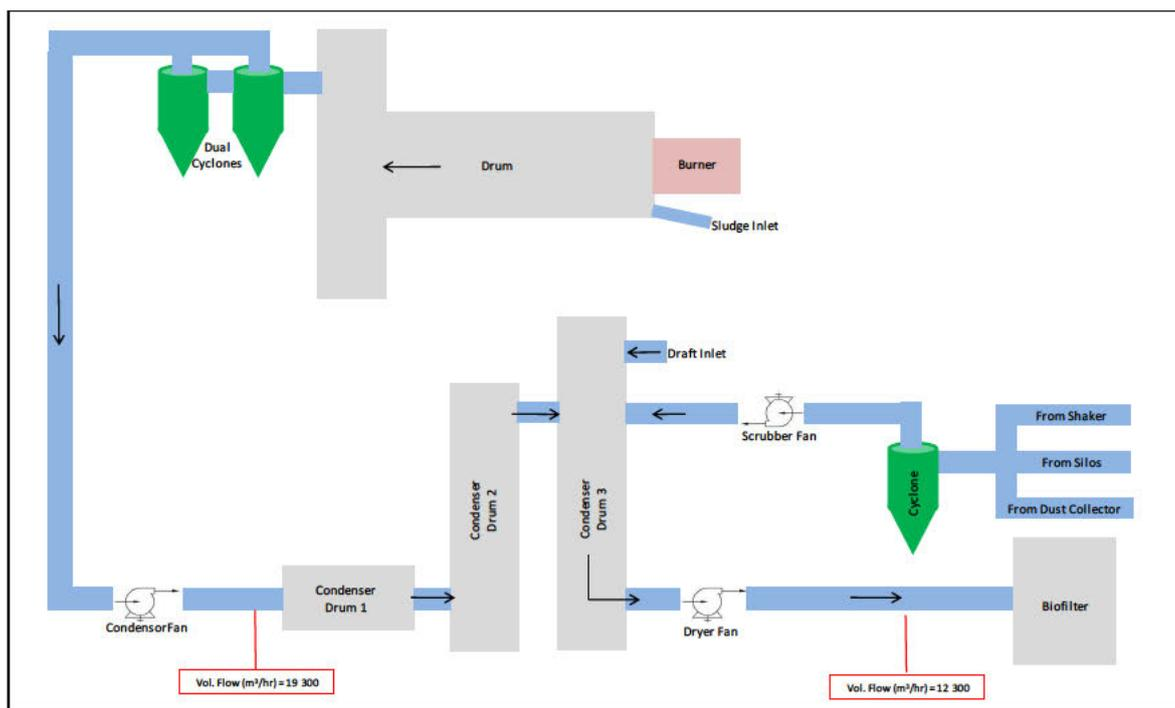
■ Figure 10: Sludge Dryer Extraction Rate Schematic, 24 February 2023
