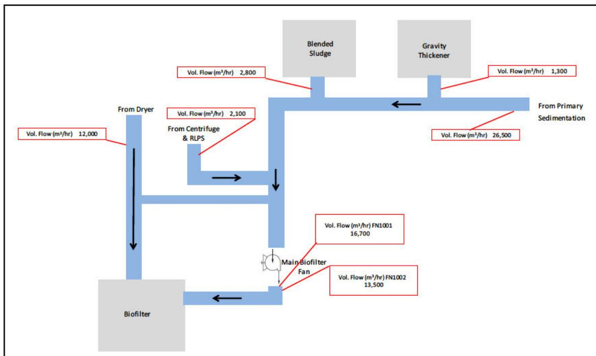
■ **Figure 10: Biofilter Total Extraction Rate Schematic, July 2021**
