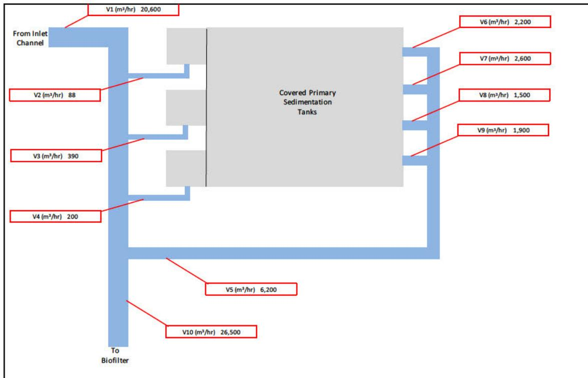
■ **Figure 7: Primary Sedimentation Extraction Rate, July 2021**
