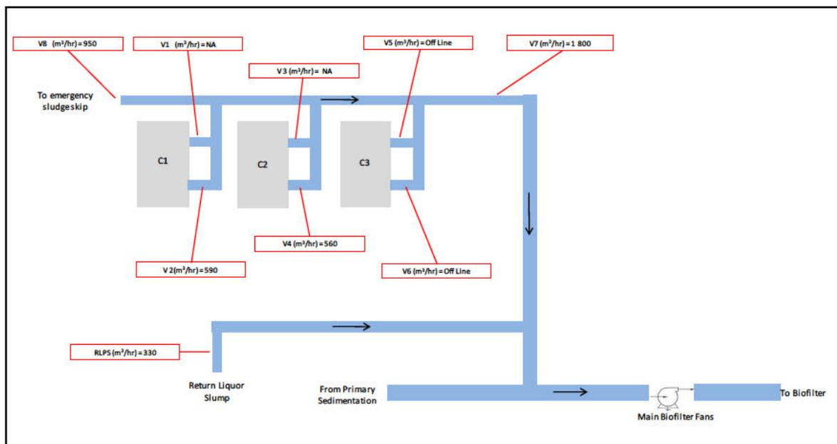
■ **Figure 8: Centrifuge Room & Return Liquor Pump Station Extraction Rate, July 2021**
