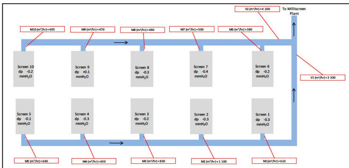
■ **Figure 5: Milliscreen (First Floor) Extraction Rates, 2 July 2021**
