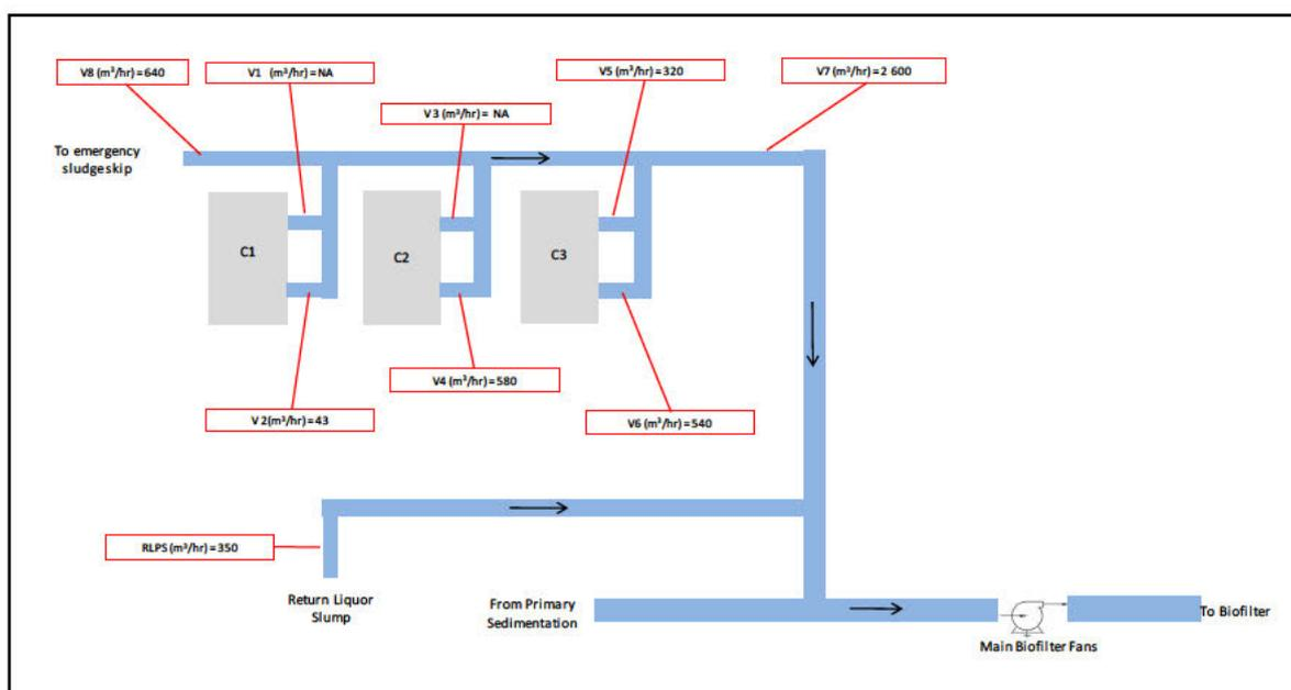
■ **Figure 9: Centrifuge Room & Return Liquor Pump Station Extraction Rate, 24 February 2023**
