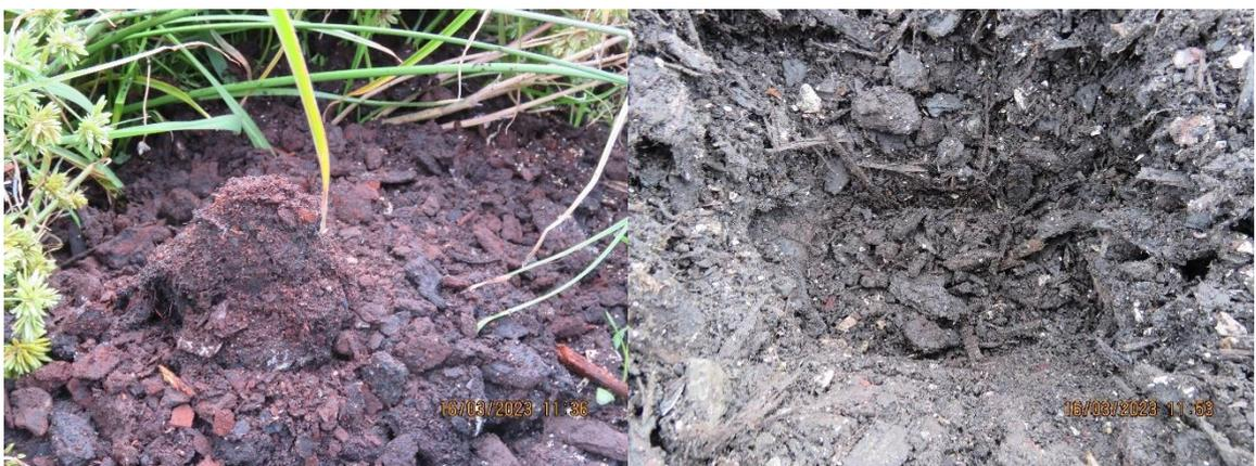
■ **Figure 7: Biofilter Media 750 mm depth – Dry and Mouldy Media, 16 March 2023**
