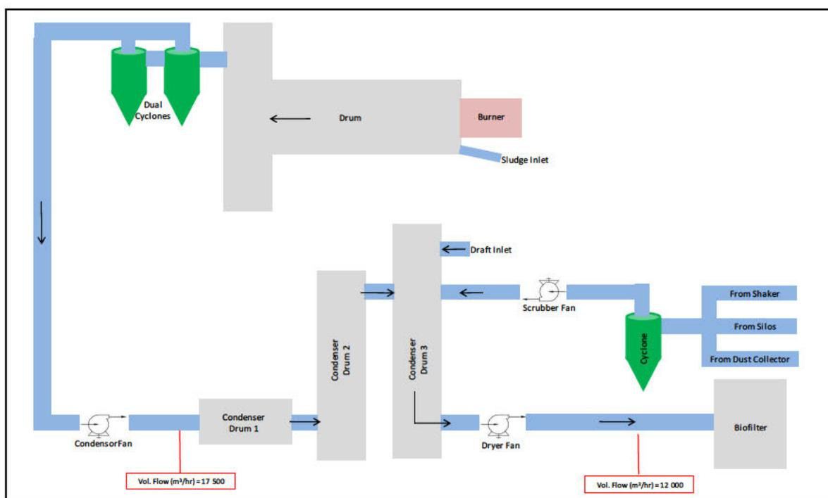
■ **Figure 9: Sludge Dryer Extraction Rate Schematic, 20 July 2021**
