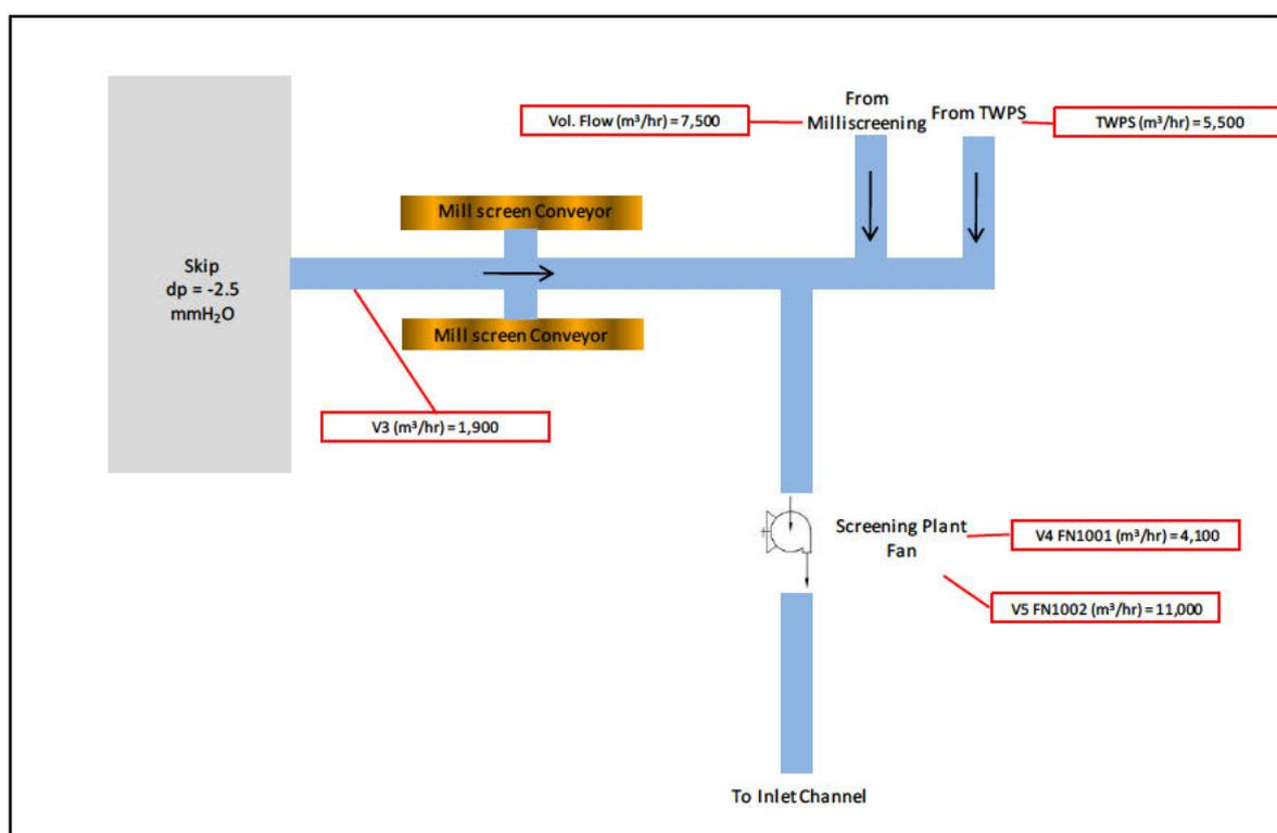
**Figure 6: Milliscreen Plant (Ground Floor) Extraction Rate, July 2021**
