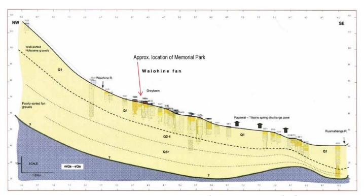
Figure 4: Greytown-Waiohine geological cross section showing fault lines and aquifer (source: Gyopari and McAlister (2010), Wairarapa Valley groundwater resource investigation: Middle Valley catchment hydrogeology and modelling. Greater Wellington Regional Council, Technical Publication No GW/EMI-T-10/73)
